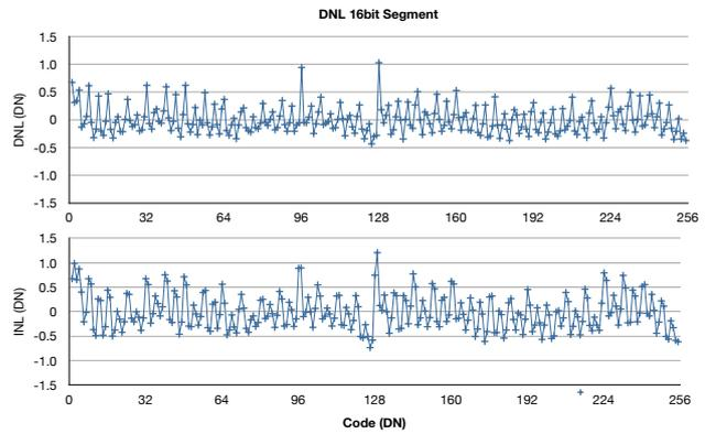
Figure 6. DNL and INL of 16bit Segment
