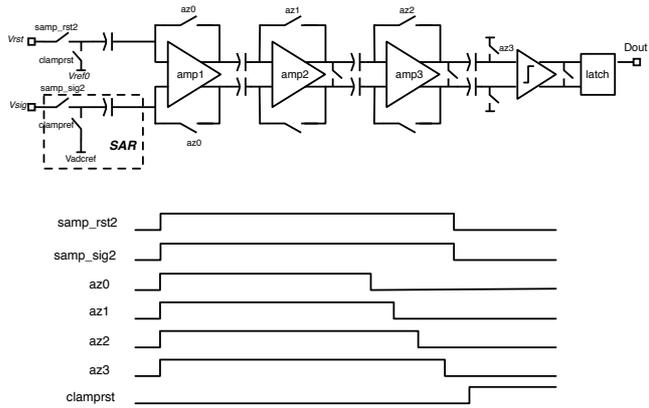
Figure 3. High Gain Comparator
