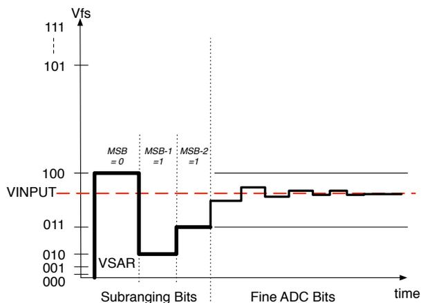
Figure 2. ADC Conversion Process
